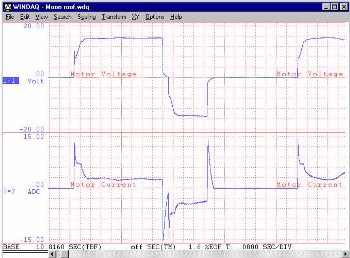
Figure 1 – A typical output from WinDaq software (shown here at a compression factor of 2) when connected to the moon roof motor through DI-730 data acquisition hardware. Notice the spikes on the current waveform that were virtually hidden on the strip chart recorder output.
