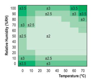
Relative humidity sensor typical and maximum tolerance at 25°
