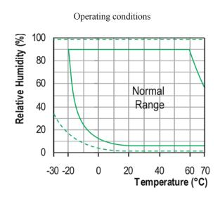
Long term exposure to humidity levels outside of the 'normal' range may temporarily offset RH measurements ( $\pm 3\%$ RH after 60 hours). Once returned to less extreme conditions the device will slowly return to a calibrated state.
