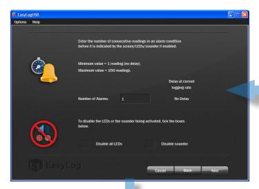
Configure alarm delay time and methods
