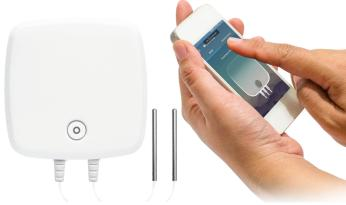
The EL-MOTE-DTP kit has been designed to monitor temperature in a large range of applications, using 75mm length barrel temperature probes on 3m cables. Ideal for monitoring locations perhaps difficult or inhospitable to the data logger itself, the EL-MOTE-DTP is ideal for monitoring refrigeration or storage units. This kit has 2 channels to monitor 2 separate areas simultaneously, perhaps a fridge and freezer.
