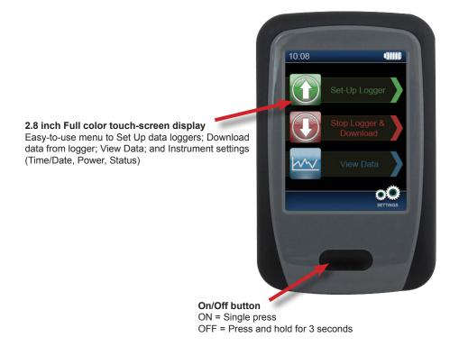
The EL-DataPad allows users of certain EL-USB data loggers to configure their units, upload data, and view logging results on-thespot rather than moving the logger to their PC. This allows shorter breaks in data collection for more data continuity, less travel time, and on-the-spot data review and data logger reconfiguration.
