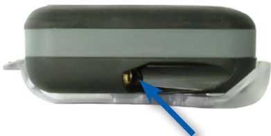
Port for Temperature Probes
