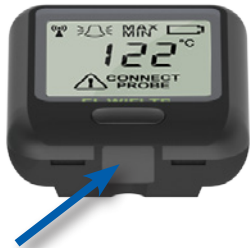
USB port sealed with rubber gasket
