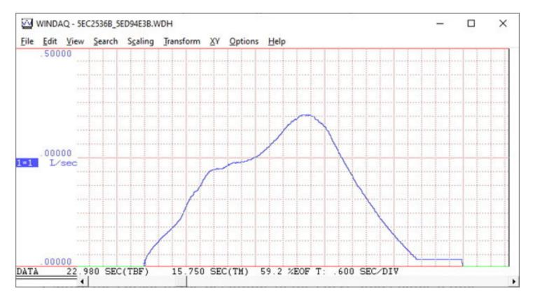
Note that connection and configuration for the WINGONEER YF-S201 Flow Sensor is the same for all contemporary DATAQ data loggers, including but not limited to the DI-2108-P, DI-2008 and DI-4108/4208. All feature a Rate channel Use comparable settings for setup in Stand-alone mode.
