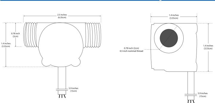
YF-S201 Flow Sensor Dimensional Drawing
