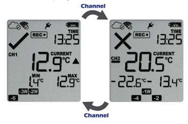
The Alarm and OK symbols are independently shown for each channel. The red LED, however, blinks as long as either channel has registered an active alarm, and the buzzer will continue to operate.
