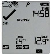
• keep holding the button after **STOPPED** remains permanently on until the **REC**• symbol reappears.
