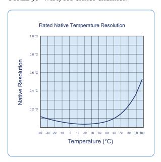
Figure 10: Rated Temperature Resolution Chart
