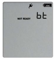
If the display does not show **bE**, you can activate the Bluetooth function by pressing and holding the **Channel/FUNCTION** button until **bE** appears.
