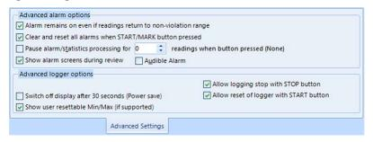
Figure 7: UTRED30-WiFi advanced configuration screen in LogTag® Analyzer 3
