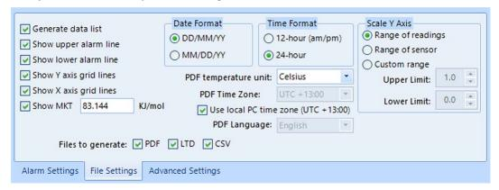
Figure 6: UTRED30-WiFi File settings screen in LogTag® Analyzer 3
