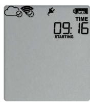
Once **READY** disappears, release the button within two seconds. **STARTING** will now disappear, and the **REC•** symbol will be shown. The UTRED30-WiFi now records temperature data.
