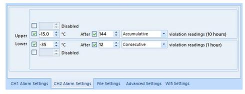
Figure 5: Sample Alarm Configuration Settings for channel 2
