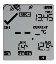
When evaluating data, any readings taken while the probe is disconnected are shown as --\_- in the data list. The chart in LogTag<sup>®</sup> Analyzer and in LogTag<sup>®</sup> Online will show a gap during this period. Minimum and Maximum values shown on the display will remain visible and will not be updated until the sensor is plugged back in.
