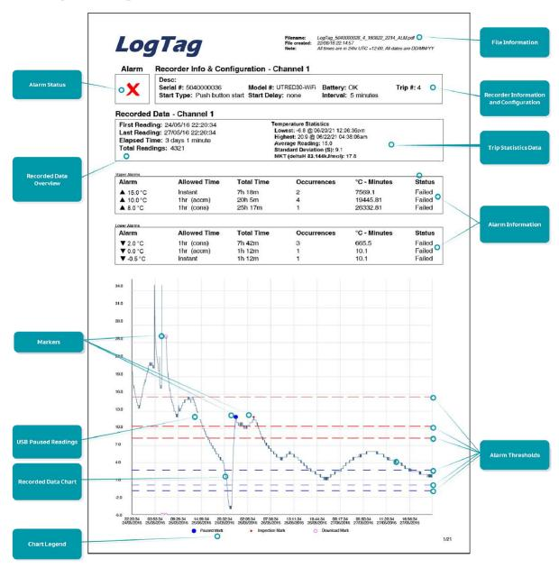
Figure 8: Sample report page with Multiple Alarm Thresholds
