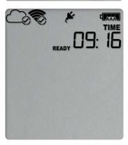
If the button is released while **STOPPED** is still , or you wait until the **READY** symbol disappears, the display shows **STOPPED** again, and the logger remains stopped. This means, the data from the previous trip is still accessible.
