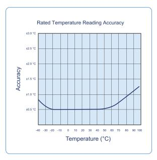
Figure 9: Rated Temperature Accuracy Chart
