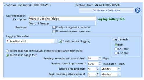
Figure 3: Standard configuration parameters for a UTRED30-WiFi
