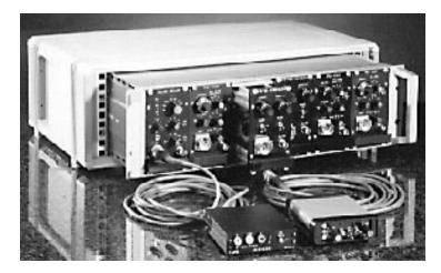
Desktop enclosure (DTE-1000) housing CC-1000 amplifier cage. Six plug-in amplifiers fully populate the CC-1000.
